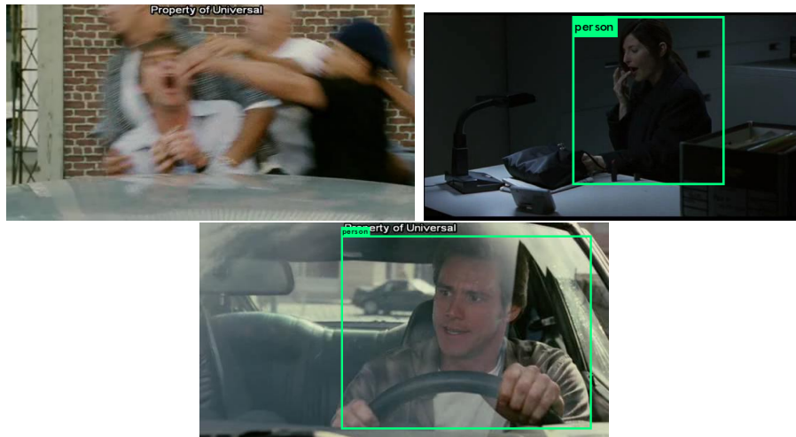
Fig. 4.8. Examples of human detection using YOLO algorithm from Hollywood2 dataset. We can observe that YOLO fails to detect the person in the first image. It successfully performs human detection in the other two images.
